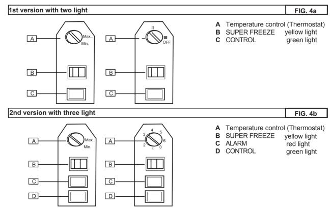
If the indicator-lights on your appliance are laid out in a different way, the following always apply: green = appliance operating; red = ALARM; yellow = SUPER FREEZE ON
